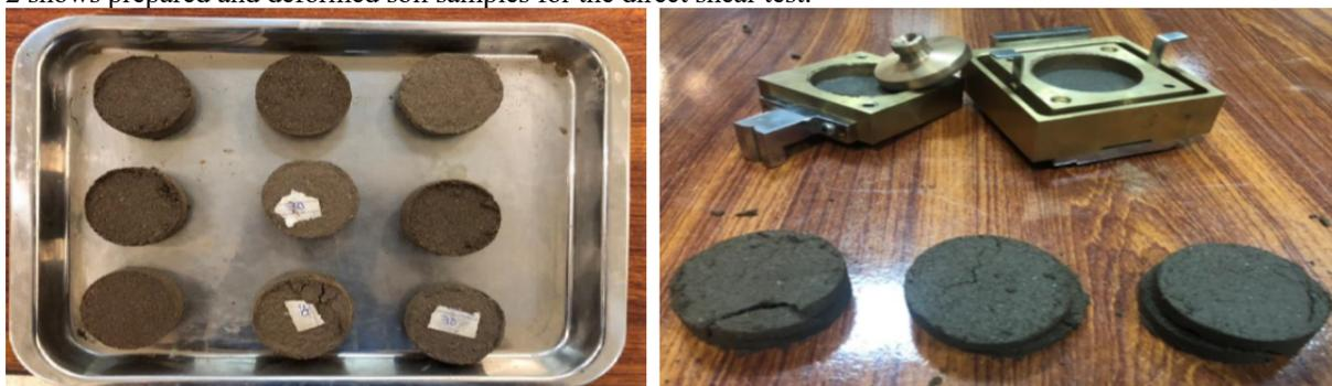
**Fig -2:** (a) Direct shear test samples; (b) Deformed direct shear test samples
