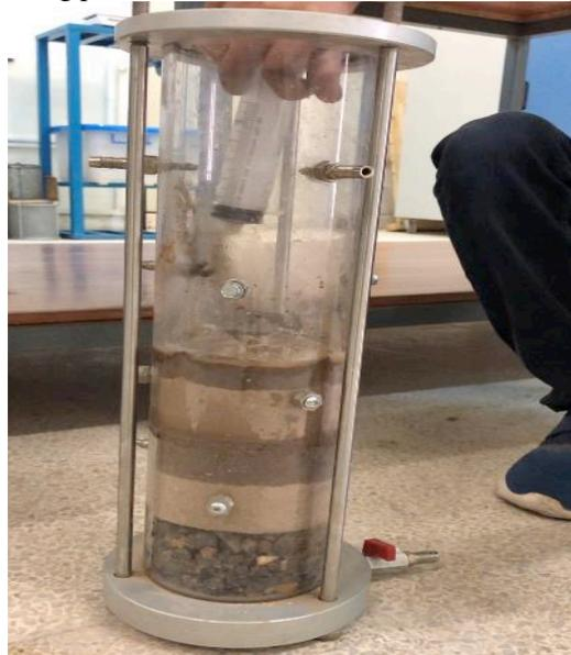
Fig -3: Injecting EICP solution into the soil
