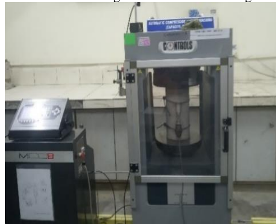
Fig 5: Test setup for Modulus of Elasticity of concrete in Strain Controlled Machine
