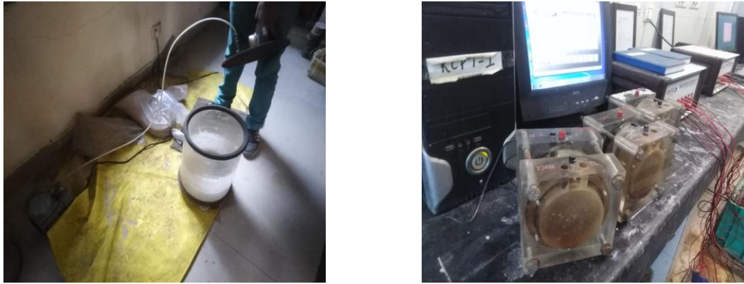
Fig -4(a): Vacuum box and 4 (b): DC voltage system for RCPT tests
