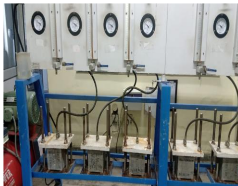
Fig -6: Test Setup for Water permeability test
