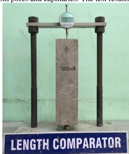
Fig -7: Test set up for Drying Shrinkage Test as per IS: 1199
