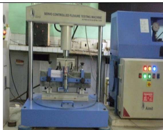
Fig -3: Sample undergoing Flexural Strength Test
