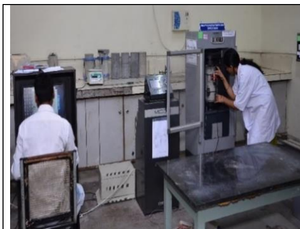
Fig -2: Test Set up for Compressive Strength Test
