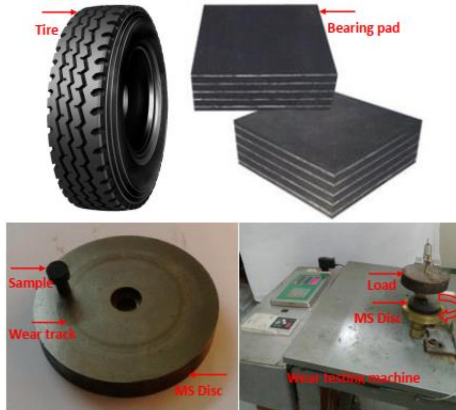
Fig -1: Experimental tire and bearing pad, wear samples, MS counter disc and Wear testing machine.
