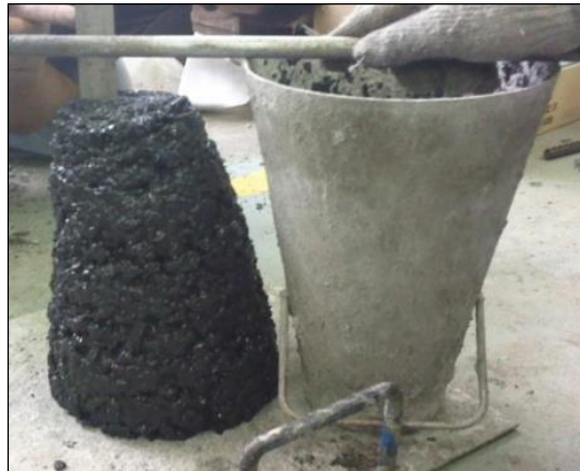
Fig - 9: Slump test [20]
