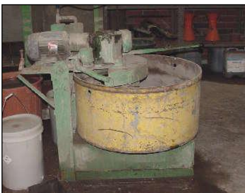
Fig -7: Mixer used in the manufacture of geopolymer [19].
