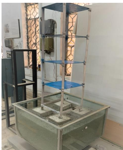
Fig. 1: Pictorial view of Frame models & isolated Footing on shake table
