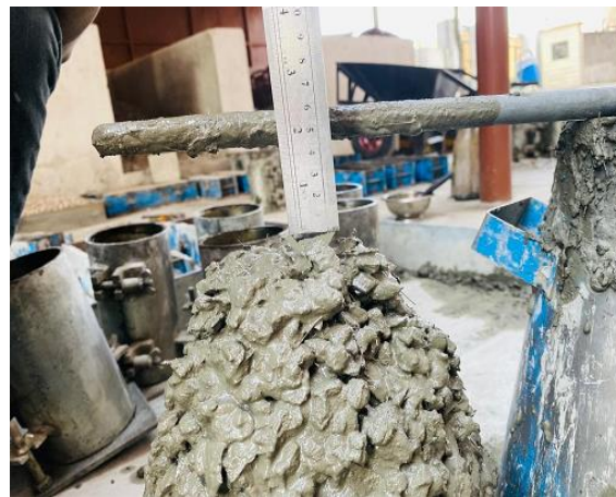
Fig-2: Slump of concrete having 15% PET particles content
