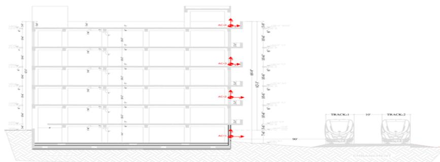
**Fig-2:** Orientation and placement of four accelerometers
