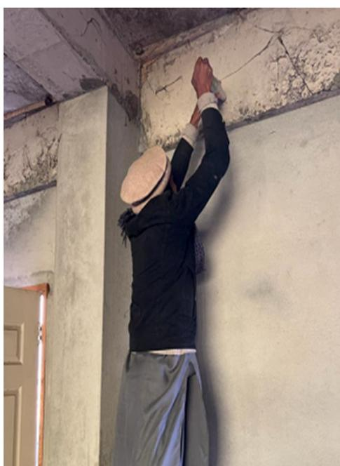
**Fig-5:** Schmidt Hammer Testing
