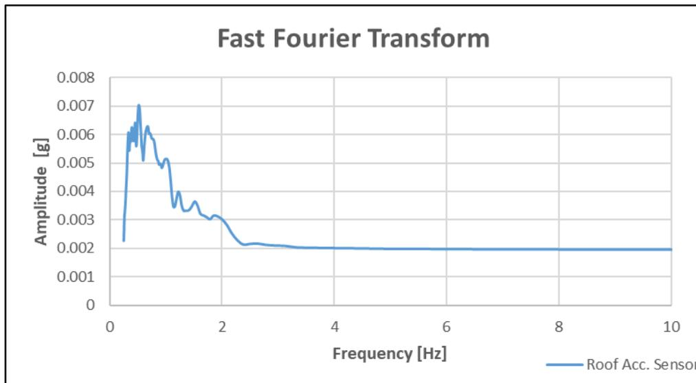
**Fig-3:** Train Induced Vibration of Building
