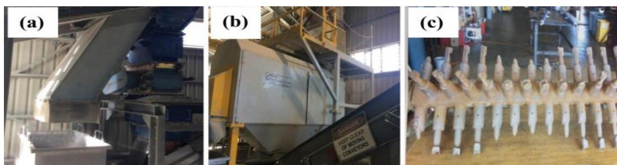
**Fig-1:** Glass crushing machine (a) Imploder (b) Shearing unit and (c) Grinding shaft [21]
