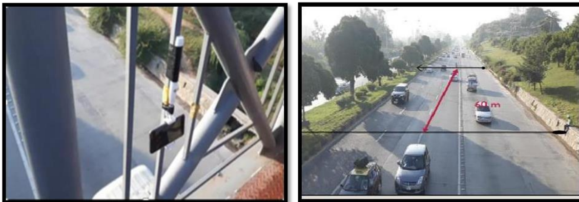
Fig-1: (Left) Fixed Camera for video at the foot over bridge, (Right) Trap length measurement
