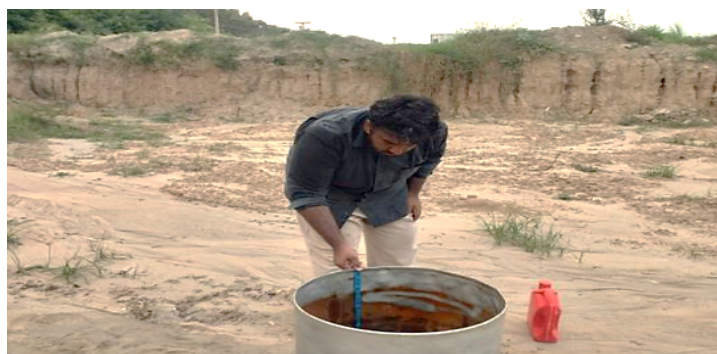
Fig-3: Single-Ring Infiltration Test
