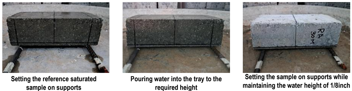
Fig-2: Testing setup of Initial rate of water absorption
