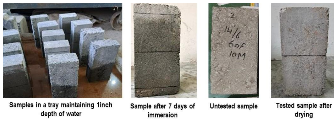
Fig- 6: Efflorescence test setup
