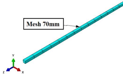
**Fig-5:** Meshing of grout
