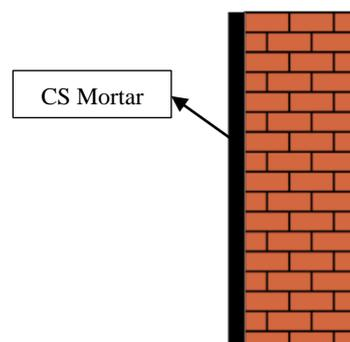
**Fig -1:** Typical details of strengthening CCIB masonry wall.
