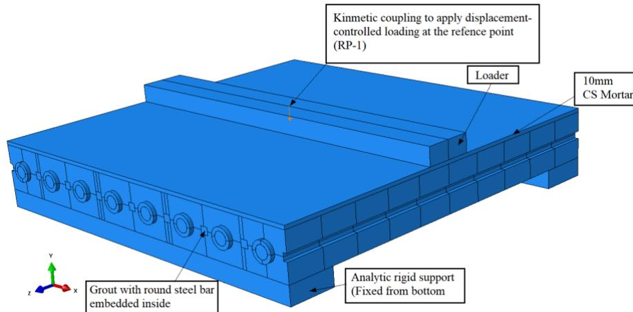
**Fig-2:** Model assembly, Loads, and boundary conditions.
