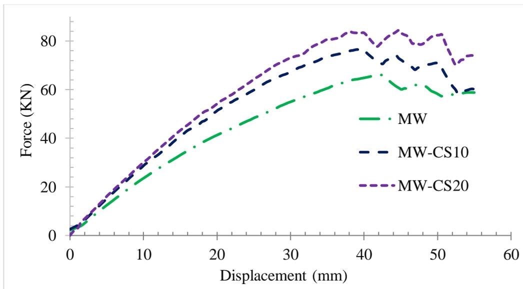
**Fig-6:** Force versus displacement responses of the CCIB masonry walls
