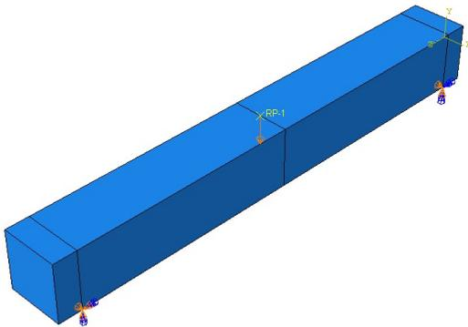
**Fig 1-c: Kinematic Coupling on the Beam.**
