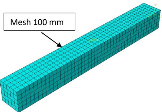
**Fig 1-d: Meshed Profile of Beam.**
