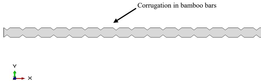
**Fig -2:** Corrugated Bamboo used for Modelling.
