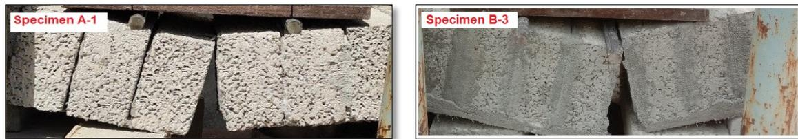
**Fig - 3:** Failure at four-point loading of (a) Un-strengthened Control block masonry beam (series-A), (b) Partially bonded tension strengthened concrete block masonry beams (series-B)
