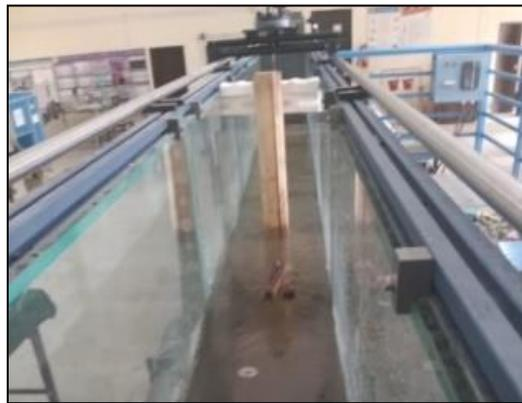
**Fig-5** Pier Fixed in Flow Channel
