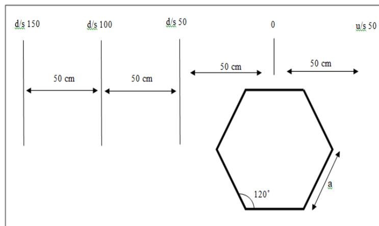
**Fig-3:** Position of Hexagonal pier along with depths at different points
