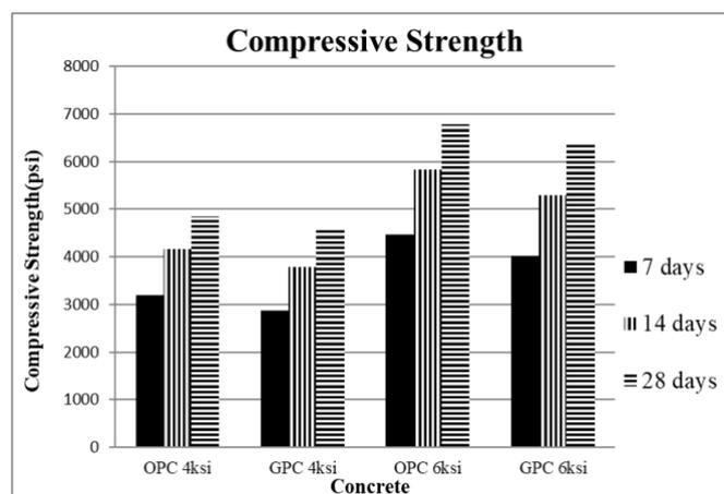
Fig -4: Compressive strength at 7, 14, 28 days
