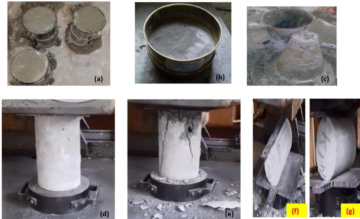
**Fig-2:** (a) Casting of concrete cylinders (b) Particle size of cement/fly ash (c) slump test (d) Compression testing (e) Compression testing (f) and (g) Split tensile testing
