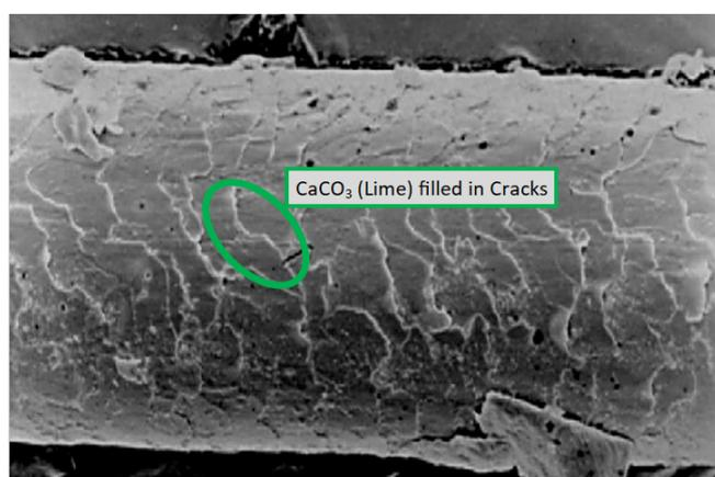
**Fig -3:** SEM Test of Healing
