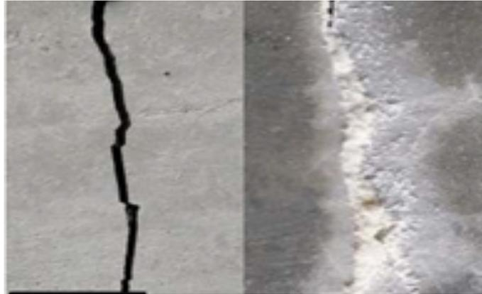
**Fig -1:** Healing of Crack [2]
