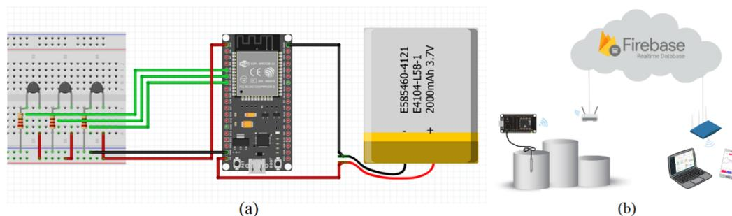
**Fig - 1:** (a) Schematic diagram of the developed sensor and (b) Overview of IoT framework
