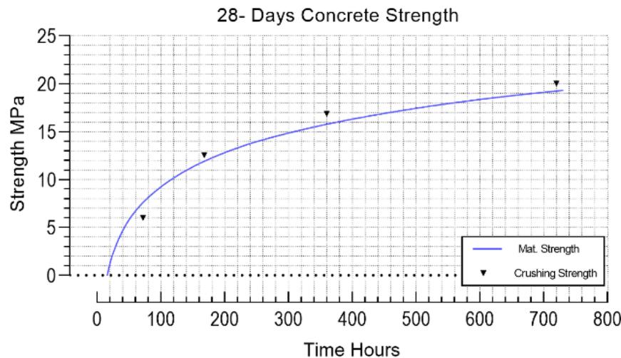
Fig - 4: Strength Comparison from Maturity Method and Uniaxial Comparison Test
