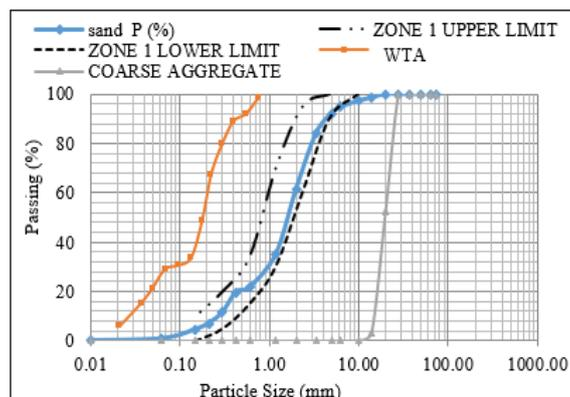
**Figure -1:** Particle size distribution of WTA, fine & coarse aggregates
