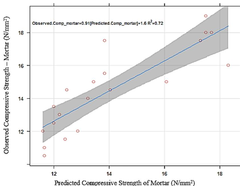
**Figure 5:** Predicted Versus Observed Values for Compressive Strength of WTA – mortar
