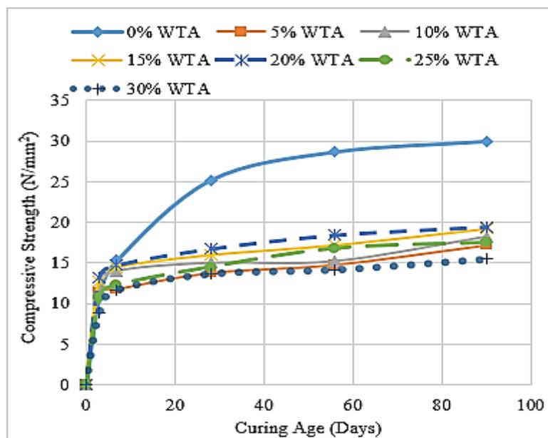
Figure 4: Compressive Strength of WTA- Mortar
